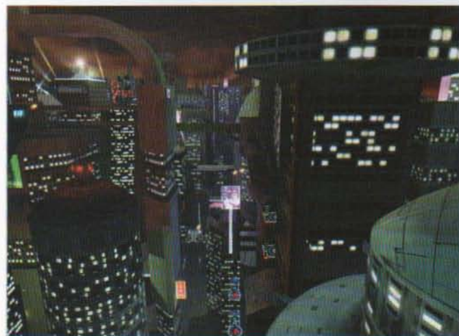
Vision engine's use of a dynamic occlusion algorithm ensures it only renders objects that can be seen from the player's viewpoint, speeding up framerates in the process
